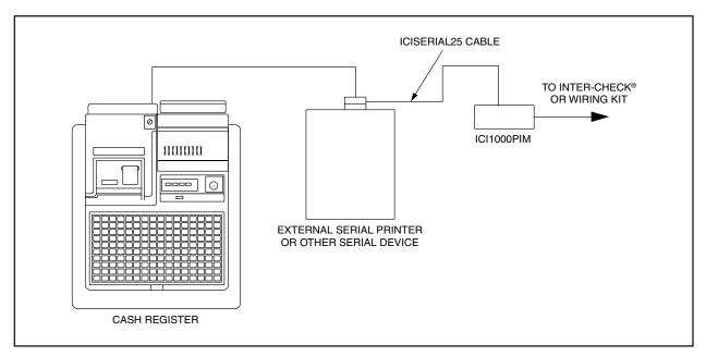
Figure 3. Interface Cable Connected to Serial Device
